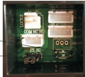
To setup the for room monitors, you must first determine the number of monitors (1-4) the system will have. If you are installing more than one room monitor, you will need to switch the jumper on the back of the monitors as noted below. This jumper has two positions. Either AF or NC. Monitors should arrive with the jumper in the AF position.
