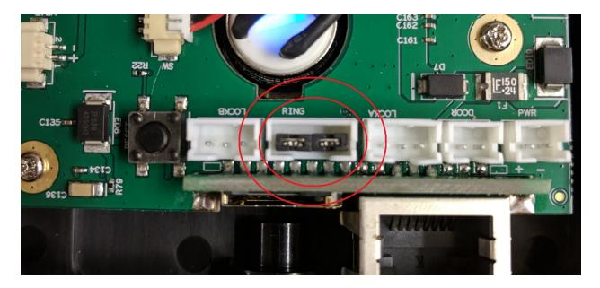
If you are *not* using the home's existing chime box and are connecting a standalone 15V transformer to power the device, the aforementioned jumpers will *not* be used. *See below.*
