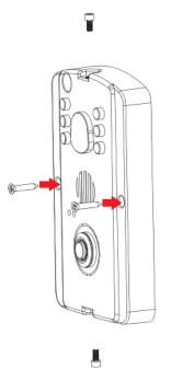
5. Lastly, position the faceplate over the MyDoor<sup>™</sup> and secure it in place with the included bolts.
