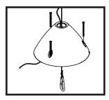
**6.** Thread cable end(s) through Gripple cable mechanisms as shown.
