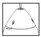
**10.** Slide cover plate over hanging and safety cables and run signal wire through center hole.
