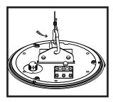
**7.** Select desired tap position. Switch is preset to maximum 70V (100V) mode.
