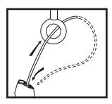
**3.** Attach snap hook by inserting one end through the hold on mounting bracket.
