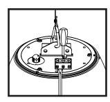
**8.** Adjust speaker hanging height with Gripple cable mechanism. Pull to tighten & press button on Gripple cable as shown to loosen or adjust.
