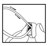
**5.** Connect signal wires to (+) and (-) inputs.
