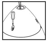
**11.** Tighten all three (3) screws to lock cover plate in place.
