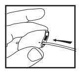
**2.** Thread hanging or safety cable through Gripple cable mechanisms as shown.
