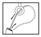
**3.** Attach snap hook by inserting one end through the hold on mounting bracket.
