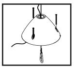
**6.** Thread cable end(s) through Gripple cable mechanisms as shown.
