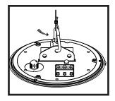
**7.** Select desired tap position. Switch is preset to maximum 70V (100V) mode.
