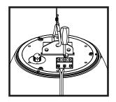
**8.** Adjust speaker hanging height with Gripple cable mechanism. Pull to tighten & press button on Gripple cable as shown to loosen or adjust.
