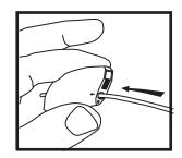
**2.** Thread hanging or safety cable through Gripple cable mechanisms as shown.
