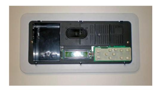
• Finish the master assembly by attaching the outer face plate and tightening the 3 screws on the bottom of the face plate.
