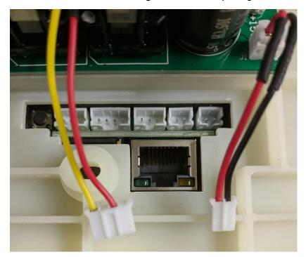
4. With all of the wiring routed *through* the opening of the adapter bracket, position it appropriately and adhere it to the wall.
