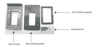
Select a height for the door station where the camera is positioned approximately eye high for the visitor. Using the rain shield as a template, mark the 4 mounting hole locations on the wall and large square hole location on the wall. In the large square you will need to drill a hole to bring the wires from inside the wall into the door station. In the 4 mounting hole locations, place 4 anchoring devices suitable for the specific wall material.
