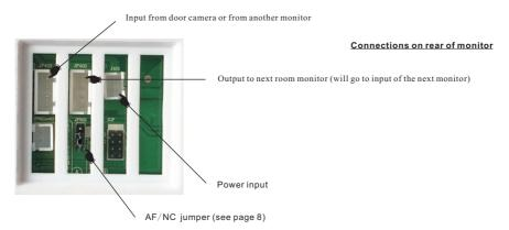
When installing more than one monitor, the monitors are "daisy chained" together. In other words, the output from one monitor is wired to the input of the next monitor. This is the same procedure for all monitors up to a maximum of 4 monitors per system.
