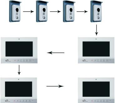
The stations are wired in series or "daisy chained" together. The output of one station goes to the input of the next station. This is done with a 4 conductor cable. Power needs to be supplied to each monitor with either the wall plug-in adapter (provided) or the opitional remote mounted power supply.
