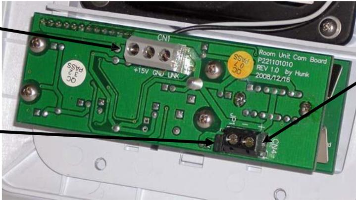
Connect external ceiling or in-wall speakers to CN4
